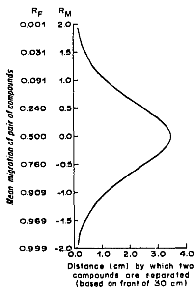
Fig. 3. Relationship between the mean migration of a pair of compounds which are separated by 0.20 R_M unit and the distance by which the compounds are separated if the solvent front is allowed to advance to 30 cm beyond the origin.
